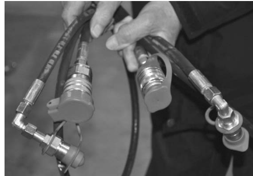
Hydraulic lines of the harvester; LH side PPV, RH side reel drive, sweeper
