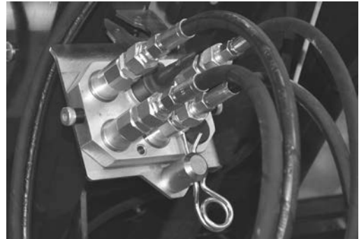
Multi-coupling on the header
