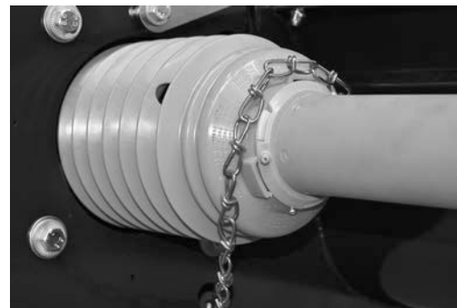
Holding chains against turning
