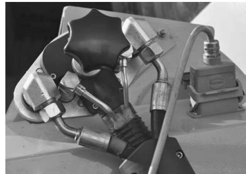
Multi-coupling on the combine harvester
