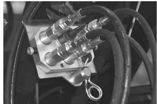
Multi-coupling on the header
