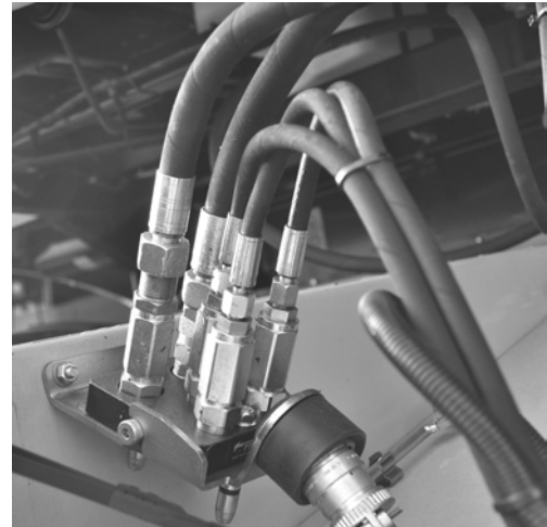
Multi-coupling on the combine harvester
