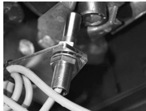
Sensor (E1) for rotational speed monitoring below the machine
