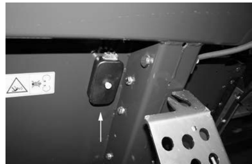
Arrow: Input additional lighting
