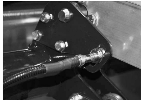
Sensor (E4) for sweeper position, backward
